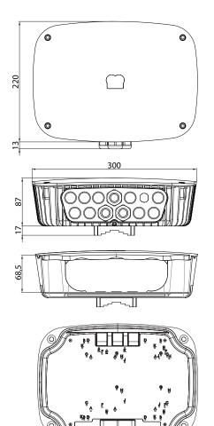
\*Data package containing Base Plate Hole Dimensions drawing and maximum inner clearance height can be found in Download list \*\*IP66 rating can be achieved by sealing the drain hole
