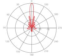
V - Port Pattern Azimuth 5.6 GHz
